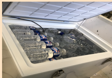
A 50W DC refrigerator on test in an environmental chamber
