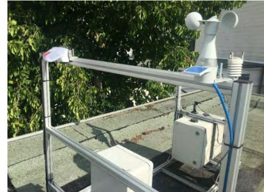
Commercial shading control devices : SOLEXA (S) and WAREMA (W).
