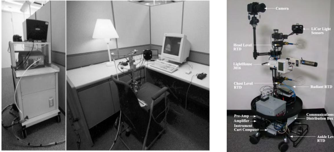
The Cart + Chair System used to generate the COPE database (NRC)
