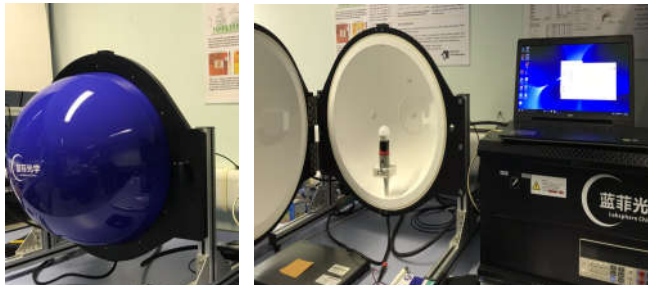
Facilities for testing of luminous efficiency of LED lighting.
