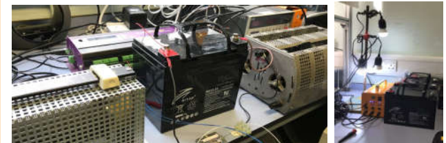
Battery discharge characterisation under various loads - appliances, resistance (left) and LED light bulbs (right)
