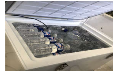
A 50W DC powered refrigerator testing in an environment chamber to understand its performance under various conditions.
